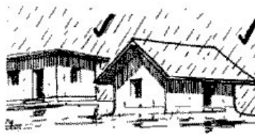
The roof MUST overhang.
