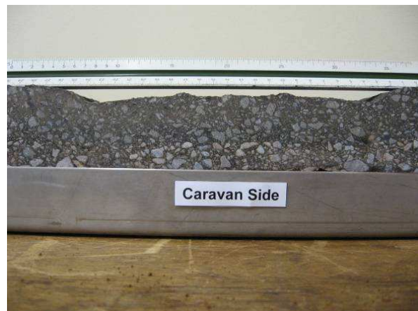
Figure 11. Typical rutting under one tyre in the HMA overlay after HVS testing in channelised mode using 60 kN and 420 kPa Inflation pressure and 60 °C (m-shape- Dual tyre loading – see Figure 9)
