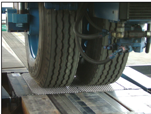
Figure 4. Dual Pad SIM system under HVS tyre testing.
