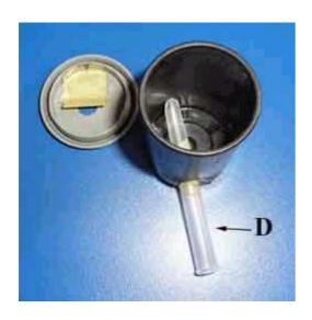
Make a hole on the cylindrical surface of (B) and press fit a gel pen old refill (D).
