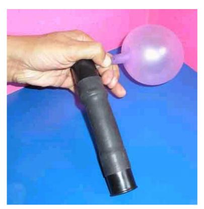
Now hold a balloon tightly to the mouth of the Delivery Pipe. Push the pull Film Can (A). The bicycle tube acts as a bellows.
