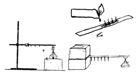
Take an iron strip approximately 15-cm long. Using a lighted candle, put a drop of molten wax on a strip about 4-cm from the end marked A. stick a 1.5-cm long nail in the wax as it cools. In this way, fix 5 more nails on the strip at 1-cm intervals. Now wedge end 'A' between two bricks with the nails pointing downwards. Heat the other end of the strip with the kerosene lamp. Record the time at which you start heating in a table. Also, record the time when each nail falls.
