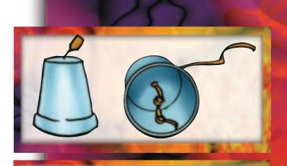
Use your thumb tack to carefully poke a hole in the centre of the bottom of a paper cup. Cut a rubber band. Thread one end through the cup and out the hole. Tie two or three knots in the end of the rubber band inside the cup as shown.
