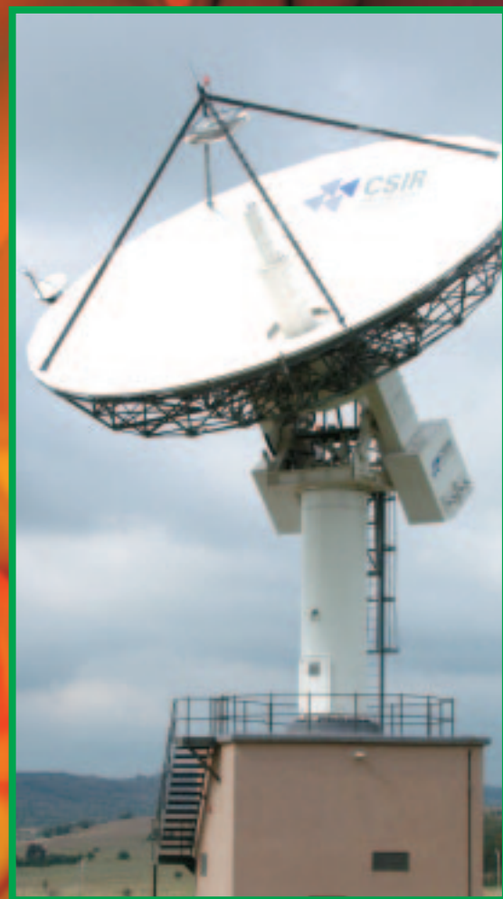
One of the CSIR SAC antennae at Hartebeesthoek. It tracks the paths of many satellites that orbit the Earth
