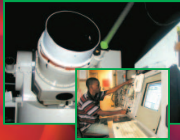
The Hartebeesthoek laser at night, with (inset) operator Sam Tshefu in action tracking a satellite
